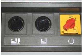
PUSH BUTTON CONTROL Push buttons allow, that the automatic clamp can be moved up and down independent of blade movement.
